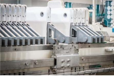
The plate-shifting mechanism allows the cake to discharge by opening each plate. The device is made up of two trolleys equipped with automatic hooks that anchor and shift the plates one by one. The trolleys move by means of toothed drive belts providing smooth and quiet operation. The belts are protected inside the trolley guide mechanism.
