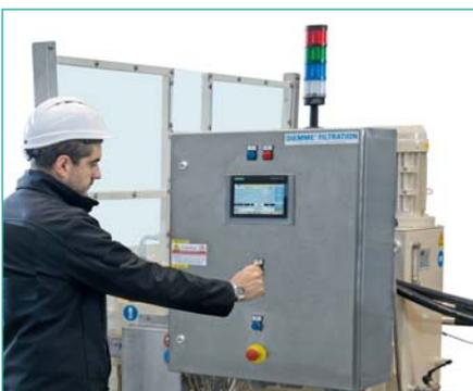
AUTOMAT filters are equipped with a PLC-based automation system with human-machine interface (HMI) that facilitates the monitoring of the filter functioning, fault diagnostics and allows the continuous adjustment of the filtration parameters in order to optimize the variable process requirements.
