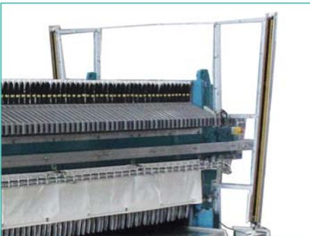
In order to maximize the accessibility of the machine and make it more user-friendly for operators and maintenance staff, we designed safety protections comprising of fixed barriers on the headers and light curtains that allow the operator to laterally access the plate pack without stopping the machine.
